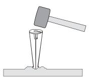
Pound mounting stake into ground with rubber mallet. Use trenching shovel if needed.
