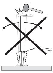
WARNING: DO NOT FORCE THE FIXTURE INTO THE GROUND
