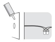
3 Mount and caulk the fixture into place, connect to homerun wire using ALOCs.
