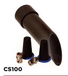
Buried connection point for central point (spider) wiring. Includes two brass connectors with set screws and plastic lug caps in PVC housing. When installed: 2.5" diameter x 9.15" depth. for direct-burial, outdoor applications. Do not use underwater.
