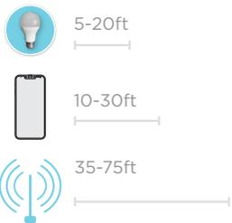
**5) Communication Distances.** bt fixtures have a Bluetooth® range of 5-20 feet in optimal conditions and bt range extenders have a Bluetooth® range of 35-75 feet in optimal conditions. Smart phones have a Bluetooth® range of 10-30 feet in optimal conditions. Bluetooth® range is affected by natural obstacles including elevation, rocks and foliage, as well as buildings, hardscapes, patio covers, and interference from other electrical (pool equipment) and wireless devices.
