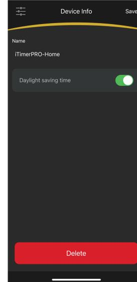
Create a custom name for the itimerPRO and toggle Daylight Savings Time on/off.
