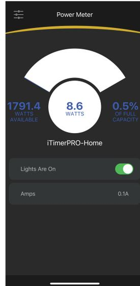
The itimerPRO has a built in power meter that will display the available capacity and the wattage and amperage consumed.
