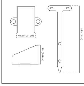
With optional glare shield and stainless steel stake
